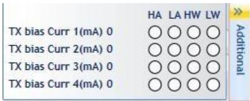
Displays the Tx bias current of the 4 channels with the HA/LA/HW/LW flags.
