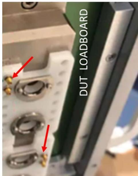
Figure 3: SMPM male connectors on loadboard blindmate connectors
